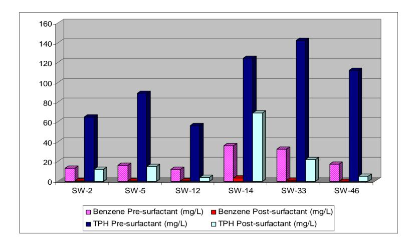
A 60-day surfactant flushing (injected 190,000 gallons of co-sufactant mixture) achieved all project goals for free-phase gasoline removal and benzene concentration reduction in ground water.
