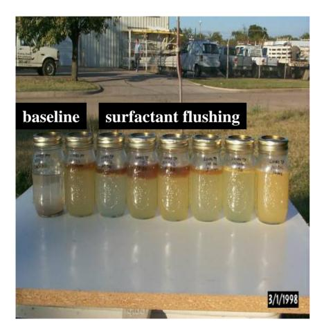
Baseline ground water(1<sup>st</sup> bottle) show no free-phase (FP) of gasoline or diesel. The ground water was collected before the surfactant flushing. **Remobilization of free-phase** gasoline and diesel during surfactant flushing (from the 2<sup>nd</sup> bottle to 8<sup>th</sup> bottle.) The FP amounts increased to a maximum (4<sup>th</sup> bottle), then decreased to a minimum (8<sup>th</sup> bottle).
