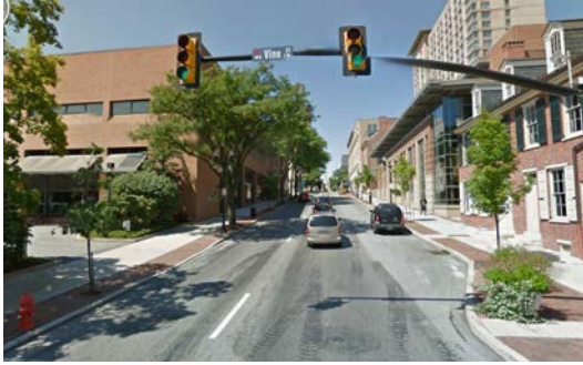
Alongside the Convention Center, Queen street's driving lanes average 15 feet wide.
