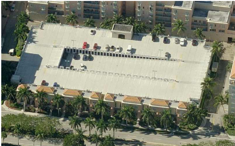
Residential apartments line the face of a parking structure in Boca Raton, FL.
