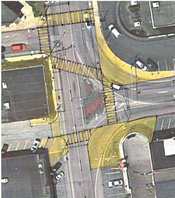
Proposed: Rectilinear corners with tight curb radii turn this back into an urban intersection. Note the two parking spaces added to the west curb.
