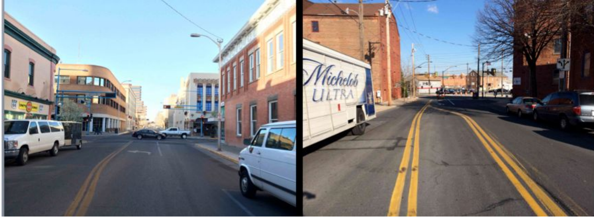
On the left, an urban left-hand turn lane, created by eliminating about 50 feet of curb parking. On the right, a highway-style left-hand turn lane on Mulberry Street, where 150 feet of parking is eliminated thanks to a mid-street no-drive zone.
