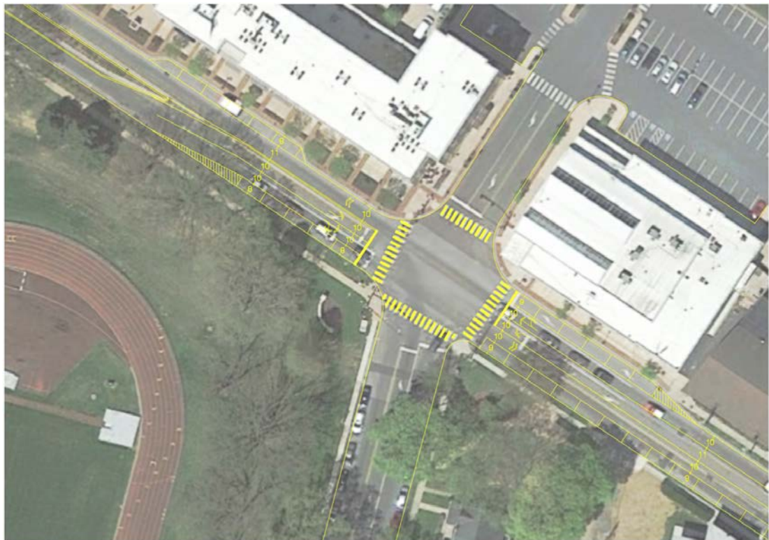
The proposed restriping right-sizes driving lanes and eliminates right-hand turn lanes, and uses the area gained to place parallel parking against curbs.
