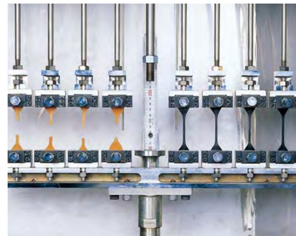
Flex fatigue test
