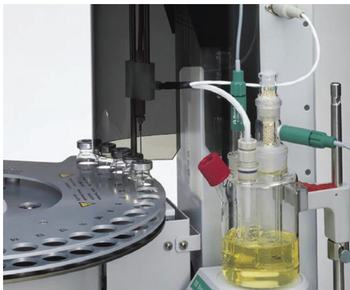
Side view of the 774 Oven Sample Processor with coulometric KF cell
