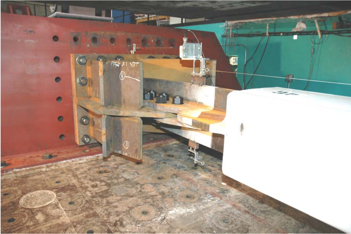
Figure 2.10 Platen End Support (East End)
