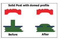
shaped heat stakes require the greatest amount of force compared to the other standard staking profiles.
