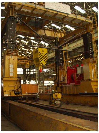
The Boiler Lift Rig:
