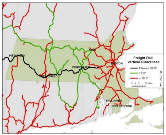
**Figure 4-5: Current Vertical Clearances**
