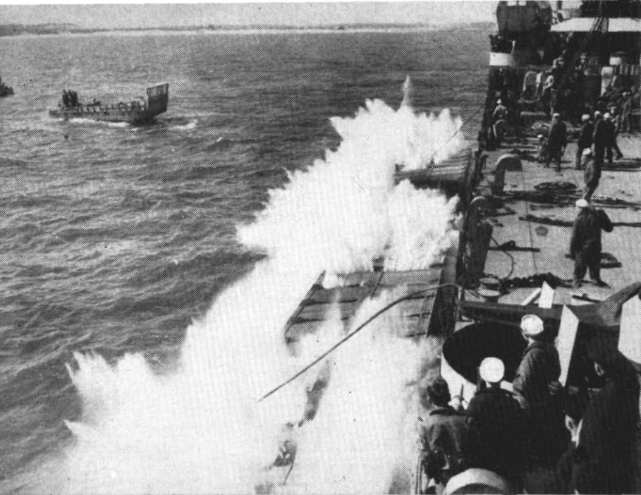
PONTOON 'string' splashes into the water as trainees learn technique of manning causeways, over which vital supplies travel from ship to shore.
