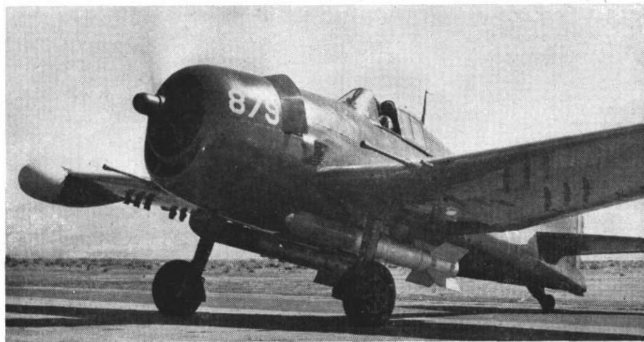
HARD-HITTING 'Tiny Tim' rockets are carried by plane preparing to take off for test. Fast-moving rocket was developed by the Navy at Inyokern.
