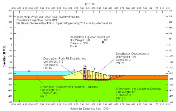
Figure 3.11 Typical cross-section of the SSA rockfill embankment.
