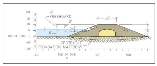
Figure 3.10 Typical Geotube® design.
