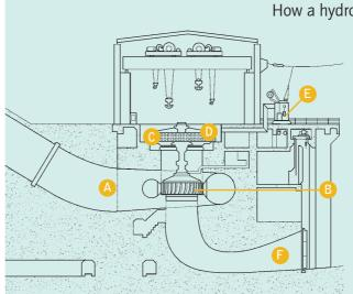
In the powerhouse, the moving water drives turbines, which in turn drive the generators connected to them. Each generator spins a shaft. On that shaft sits a part that has magnets on it which also spins – called the rotor. The rotor spins inside a part that also has magnets on it but does not move – called the stator. Having one set of spinning magnets within another set that does not move creates a magnetic field. It's this
