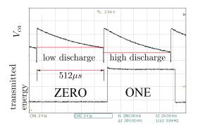
Fig. 2. LED capacitance discharge due to received light using a symbol period of  $T = 512 \,\mu$ s. At the bottom we show the signal transmitted and at the top the one received. The discharge is slower when it receives ZERO.
