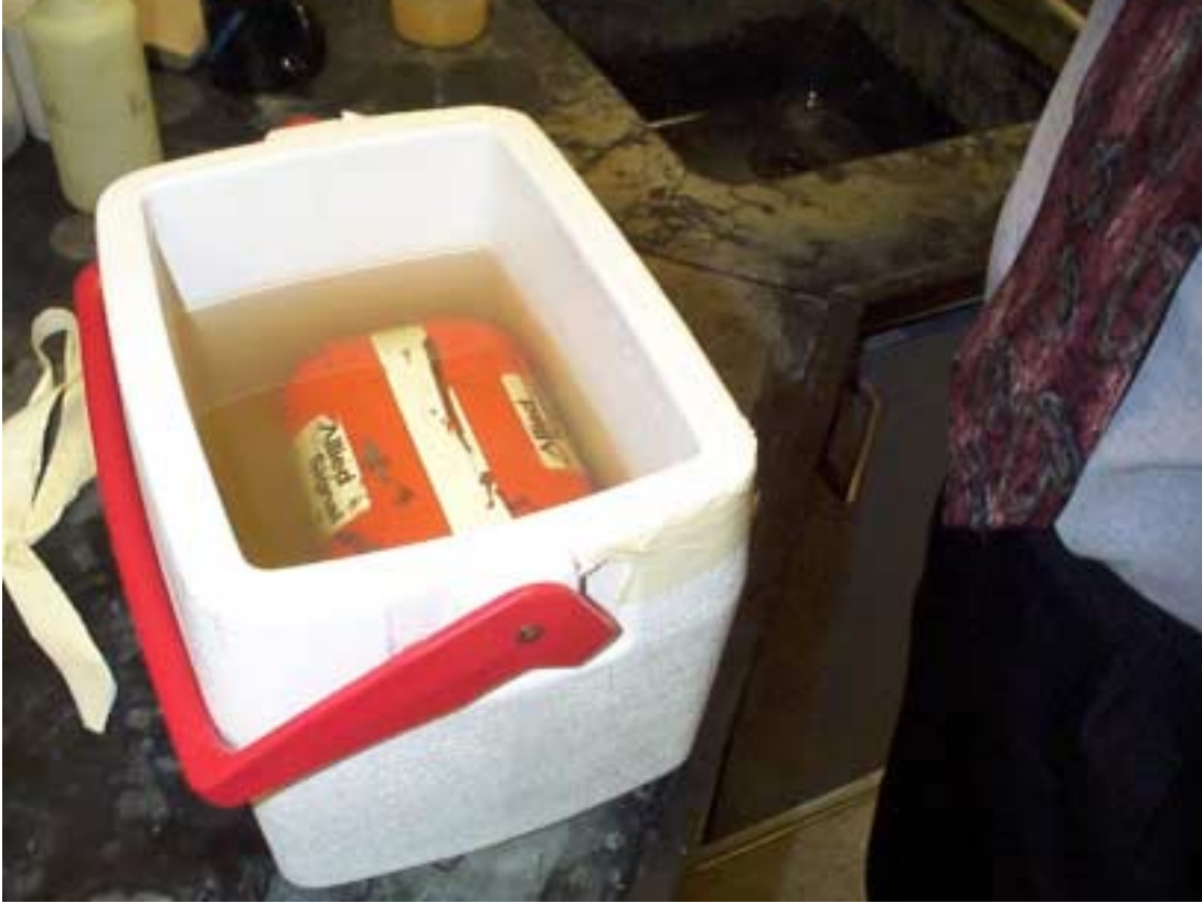
Figure 5.a Solid State CVR Module immersed in the river water
