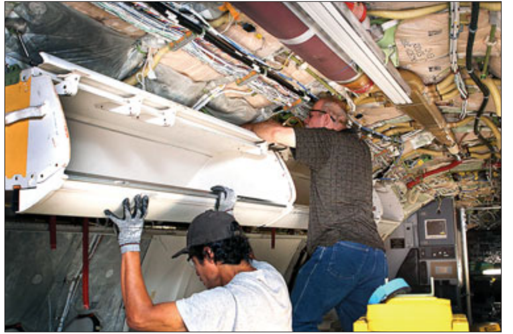
Workers install larger bins for carry-on luggage on a Boeing 737 in Tulsa, Okla.
