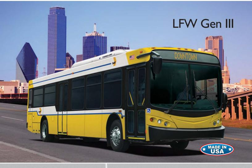
ABI's "LFW" family of low-floor buses is not a totally new product line—it just looks that way. The LFW is actually a thoroughly proven vehicle platform developed in 1999 and first Altoona tested in 2000. Since then, thousands of these venerable low-floor buses have been delivered throughout the USA, using diesel and natural gas fuels, with conventional as well as hybrid drive systems.
