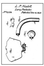
and used water moistened woolen fabric as a filtering material. It also had an exhaling valve to prevent carbon dioxide poisoning. For more "more volatile substances, such as gas, smoke, etc.," the device used a hose that moved the intake valve near to the floor.<sup>26</sup>
