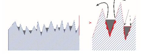
Fig. 9. Ground surface that has been significantly enlarged in the diagram. Dirt and other deposits ensure that chlorine ions, for example, are able to penetrate deeply underneath these depositions leading to local corrosion of the surface. Corrosion products such as rust will then appear.
