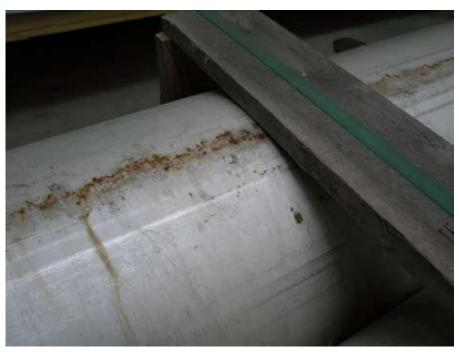
Fig. 7. Stainless steel 316 tube that was badly contaminated by steel grit on a building site.
