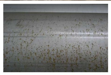
Fig. 1. contamination corrosion on stainless steel tubes caused by carbon steel grinding.
