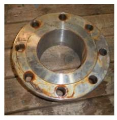
Fig. 5. RVS 304 flange contaminated by ferruginous water.
