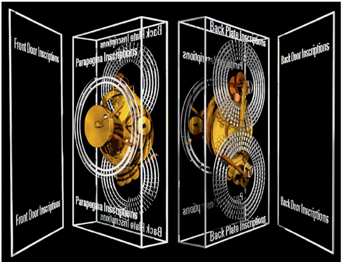
Figure 2: A schematic view of the Mechanism to illustrate the position of major inscriptions and dials. The Front Dial has two concentric scales. The inner scale shows the Greek Zodiac with 360 divisions. There are occasional Greek letters denoting references to the Parapegma inscription, and we add three further reference letters (Z, H, \Theta ) to Price's description 1 . The Parapegma is a star almanac showing rising and settings at dawn or evening of particular stars or constellations, which we will discuss elsewhere. Its form is consistent with a late 2 nd Century BC date. The outer (originally) movable scale is a Calendar carrying the Egyptian names of the months with Greek letters. The Egyptian Calendar of 365 days, with twelve 30-day months and 5 extra (epagomenai) days was in standard use in Greek astronomy. The effect of the extra quarter day in a year could be corrected by turning the scale one day every four years – and a sequence of holes to take a locking pin is observed under the scale. We find that spacing of the holes is indeed what would be expected for a total of 365 days, with a possible range 363-365. The position of the Sun and Moon would have been indicated by pointers across the dial scales, and a device 7 showing the phase of the Moon was probably carried round on the lunar pointer. It is not clear whether the Sun position pointer would have been separated from a date pointer, or whether any planetary positions might have been displayed. The spiral Upper Back Dial displays the luni-solar Metonic sequence of 235 lunar months with a subsidiary dial showing the Callippic cycle, while the spiral Lower Back Dial displays the 223 lunar month Saros eclipse cycle with a subsidiary dial showing the Exeligmos cycle.
