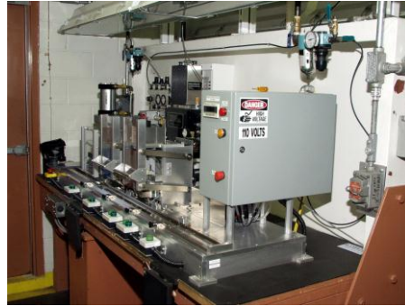
SCB Initiator Semi automated Manufacturing Line
