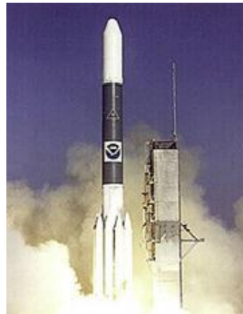
GEM and STAR Propulsion Power Delta II
