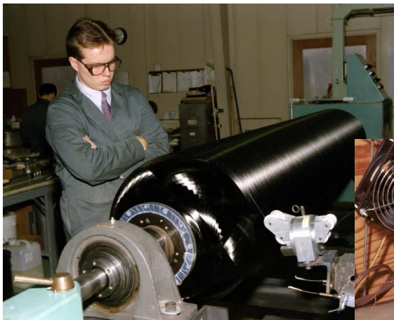
Graphite-Epoxy Composite Case Winding (21-in. booster)
