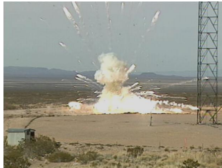
STAR 48 Destruct Test Using Model 2011 CSC
