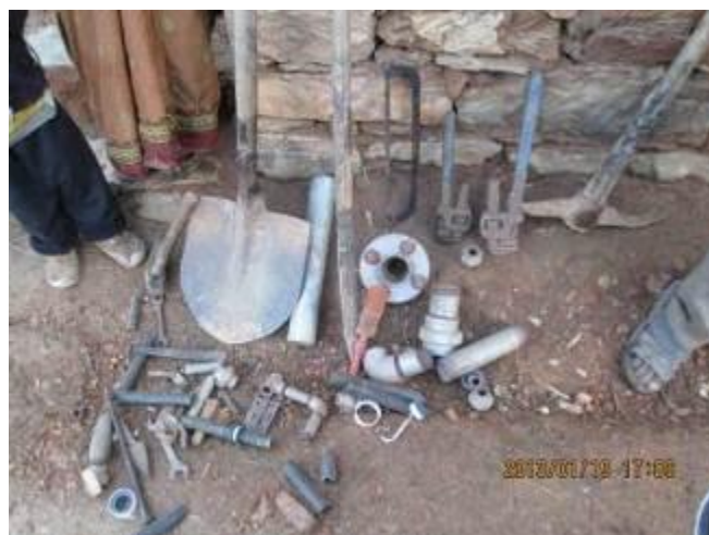
Maintenance tools and spare parts in Jhaulekh W.S.P in Siddeshwor VDC of Baitadi
