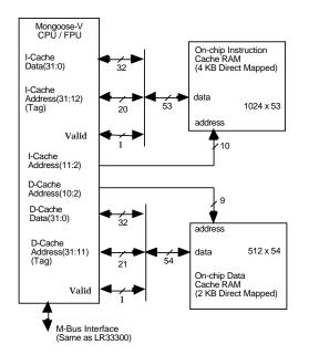
The data cache line consists of a single 32-bit data word, the valid flag and the cache tag as shown below.
