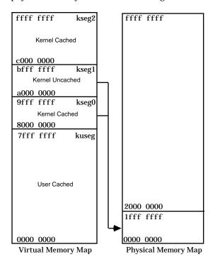
Processes executing with kernel privileges are allowed access to all four segments. Processes executing in User Mode are restricted to accessing the Kuseg only. All segments are cached except for the kseg1. In addition, kseg0 and kseg1 are hardwired to be mapped to the low 0.5 GB of physical memory. kseg2 and kuseg are directly mapped to physical memory.
