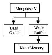
The CPU utilizes a write-through cache policy where the word written from a Store instruction is written to the data cache and also written to the write buffer. The write buffer then outputs the word to main memory when the memory becomes available. In the event that the Write Buffer becomes full, the CPU will stall when a write is pending.
