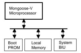
The Mongoose-V implements the MIPS R3000 instruction set including the MIPS floating point hardware. On-chip caches provide high bandwidth memory access to keep the CPU operating efficiently. The data cache size is 2 KB and the instruction cache size is 4 KB.
