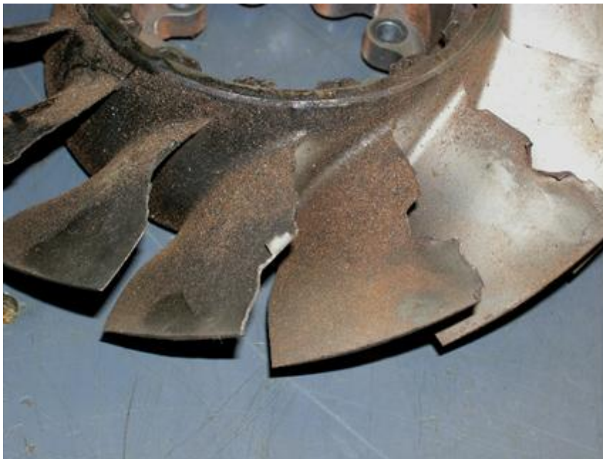
Compressor 1 st stage blades, detail
