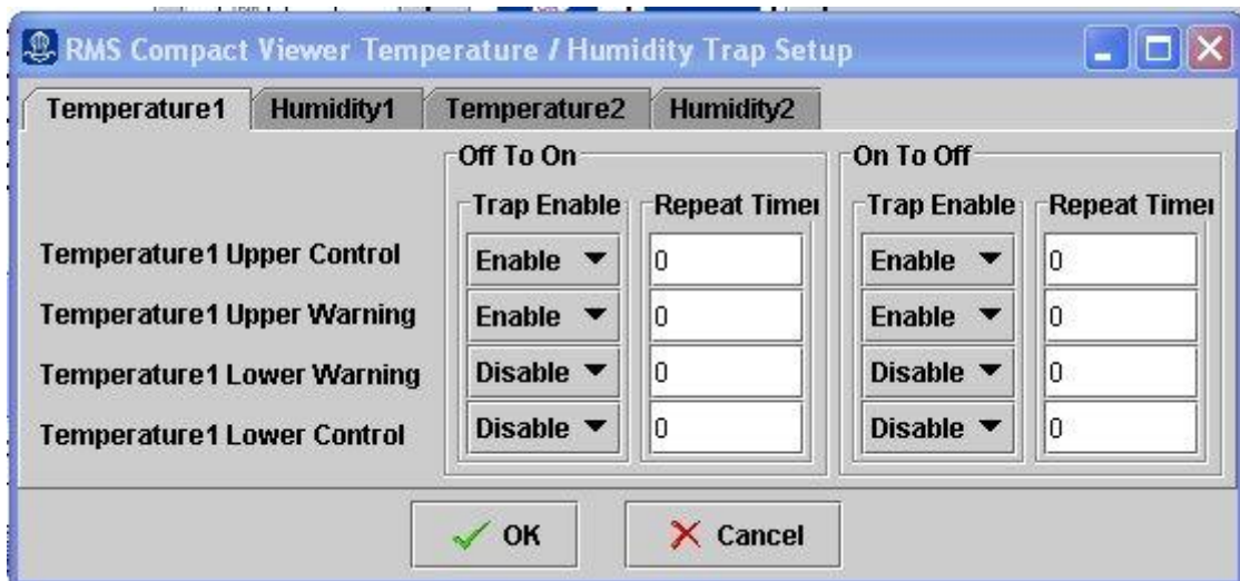
Figure 46: Temperature & Humidity Trap Configuration
