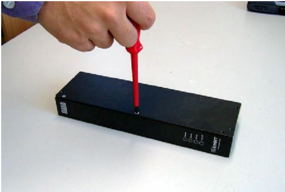
Figure 69: Removing Screws on Top of RMS Compact
