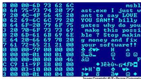
Imagen: Hex dump of the Blaster virus, showing a message left for Microsoft CEO Bill Gates by the virus programmer xi
