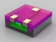
**Polishing** - scale: transistor level (~50-200nm) The excess material is polished off.
