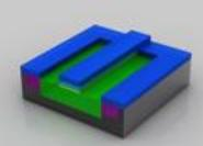
Applying Photo Resist – scale: transistor level (~50-200nm)
