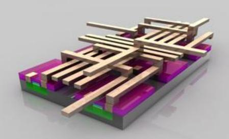
Metal Layers – scale: transistor level (six transistors combined ~500nm)
