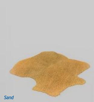
With about 25% (mass) Silicon is – after Oxygen – the second most frequent chemical element in the earth's crust. Sand – especially Quartz - has high percentages of Silicon in the form of Silicon dioxide (SiO<sub>2</sub>) and is the base ingredient for semiconductor manufacturing.
