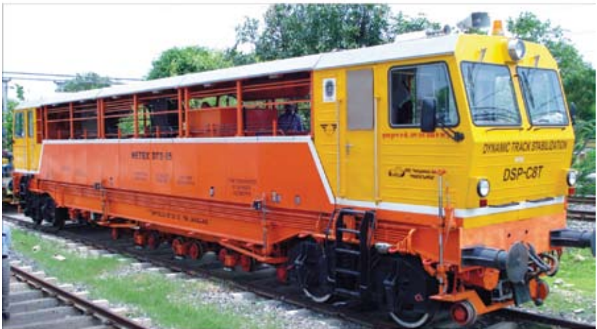
Exterior view of Dynamic Track Stabilization, North Central Railway.
