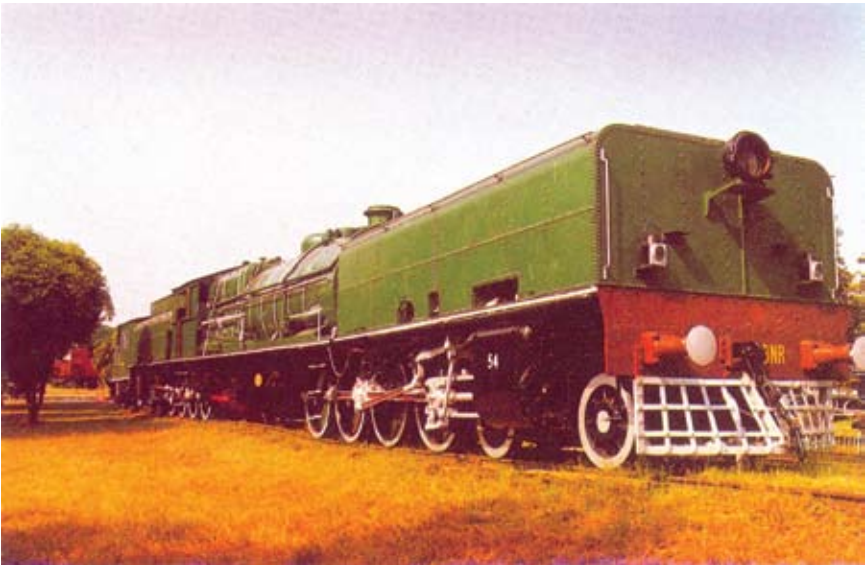
'Garratt'-built in 1930, the heaviest steam loco ever used on IR, capable of hauling 2400t on a 1 in 100 gradient.
