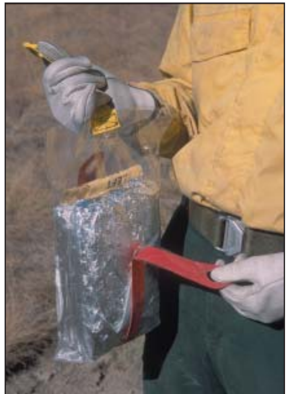
Figure 18—Pull either red ring to remove the plastic bag.
