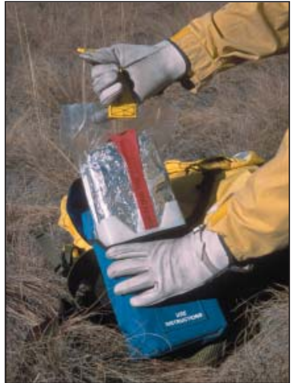
Figure 17—Use the pull strap to remove the shelter from its case.
