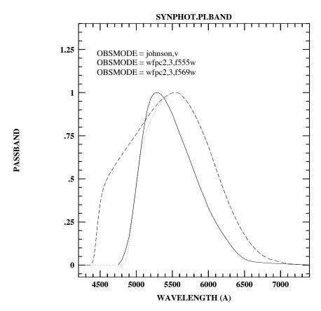
As you can see, the F569W bandpass is a closer match to Johnson *V*, especially on the blue edge. However, since the F569W bandpass is narrower than the F555W, it will have a lower overall throughput than the F555W. But how much lower? You can use the **bandpar** task to find out.
