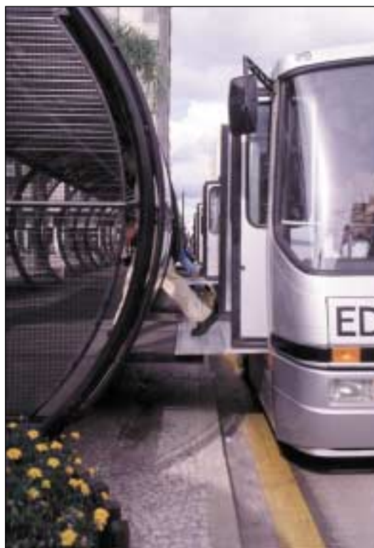
Figure 3 The direct bus has special platforms for quick docking at the tube station
