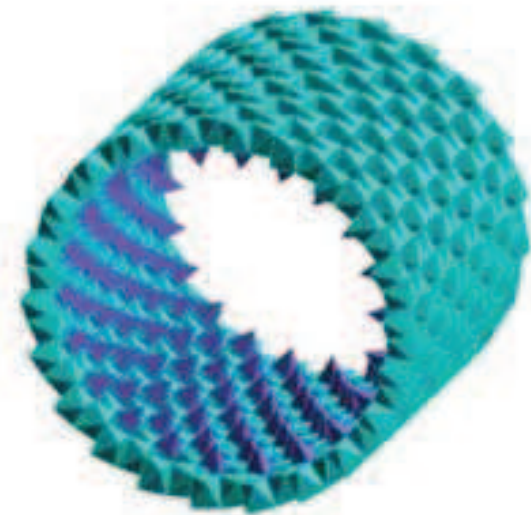
Imogolite (silico aluminates) tubes for energy storage or bumper (CEA)
