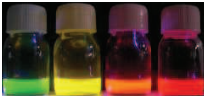
1 material (CdTe), continuous adjustable colors according to the size
