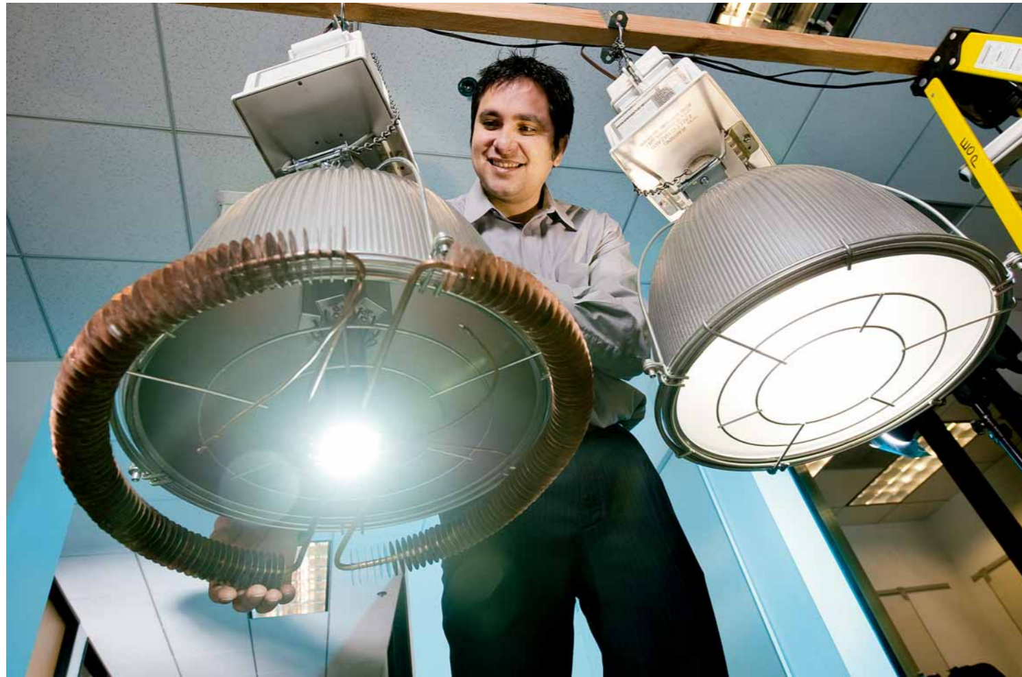
Ahmed Shuja (above) and Praveen Medis (center) have developed the world's brightest LED source (left). Rated at 15,000 lumens, it not only outshines metal halide lamps, but uses 60 percent less energy.
