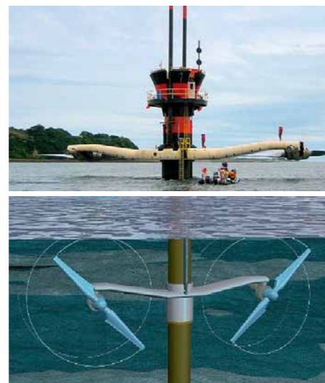
Rotors turn with the tide and produce electricity in a process developed by Marine Current Turbines.
