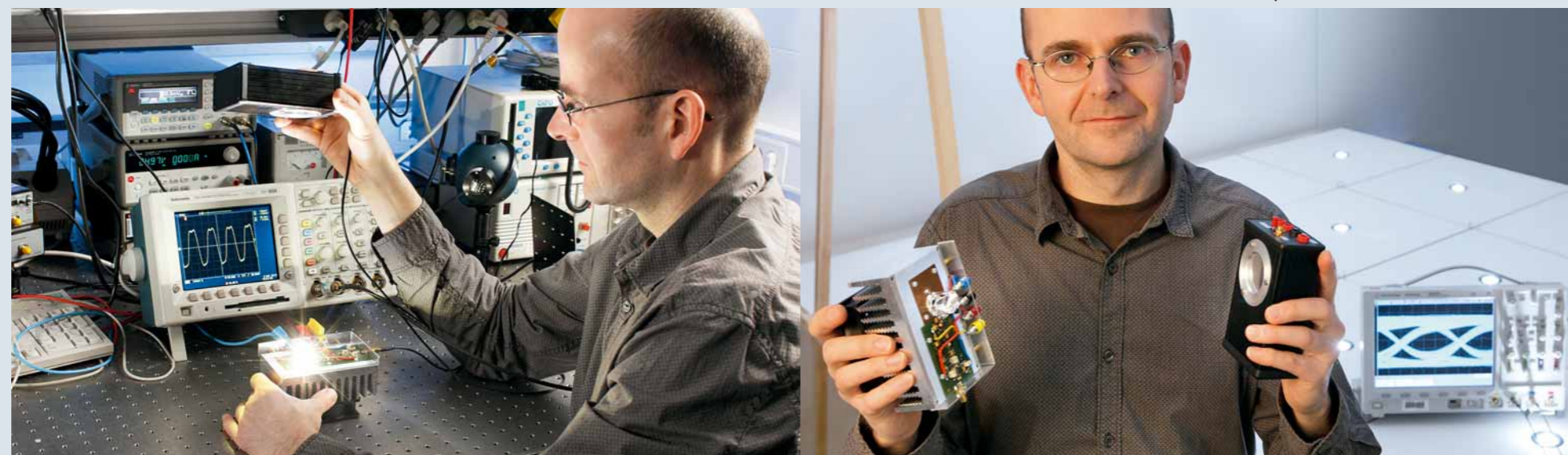
By modulating white LED light, Siemens researchers in Berlin were able to set a record for digital data transfer — 500 megabits per second over up to five meters.
