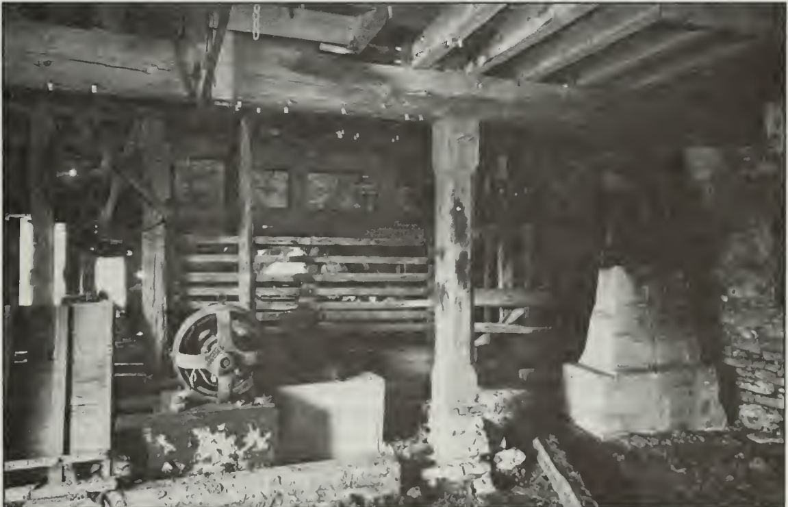
Photo 14. Huntingdon Furnace grist mill drive train, with Crocker-Wheeler generator in left foreground. Photo by Jet Lowe.
