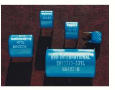
The SR Series of Surge Resistors for PCB mounting are manufactured from a carefully selected mixture of clays, alumina and carbon. After blending, the material is pressed to the required shape and then fired, in a controlled atmosphere, at high temperature.
