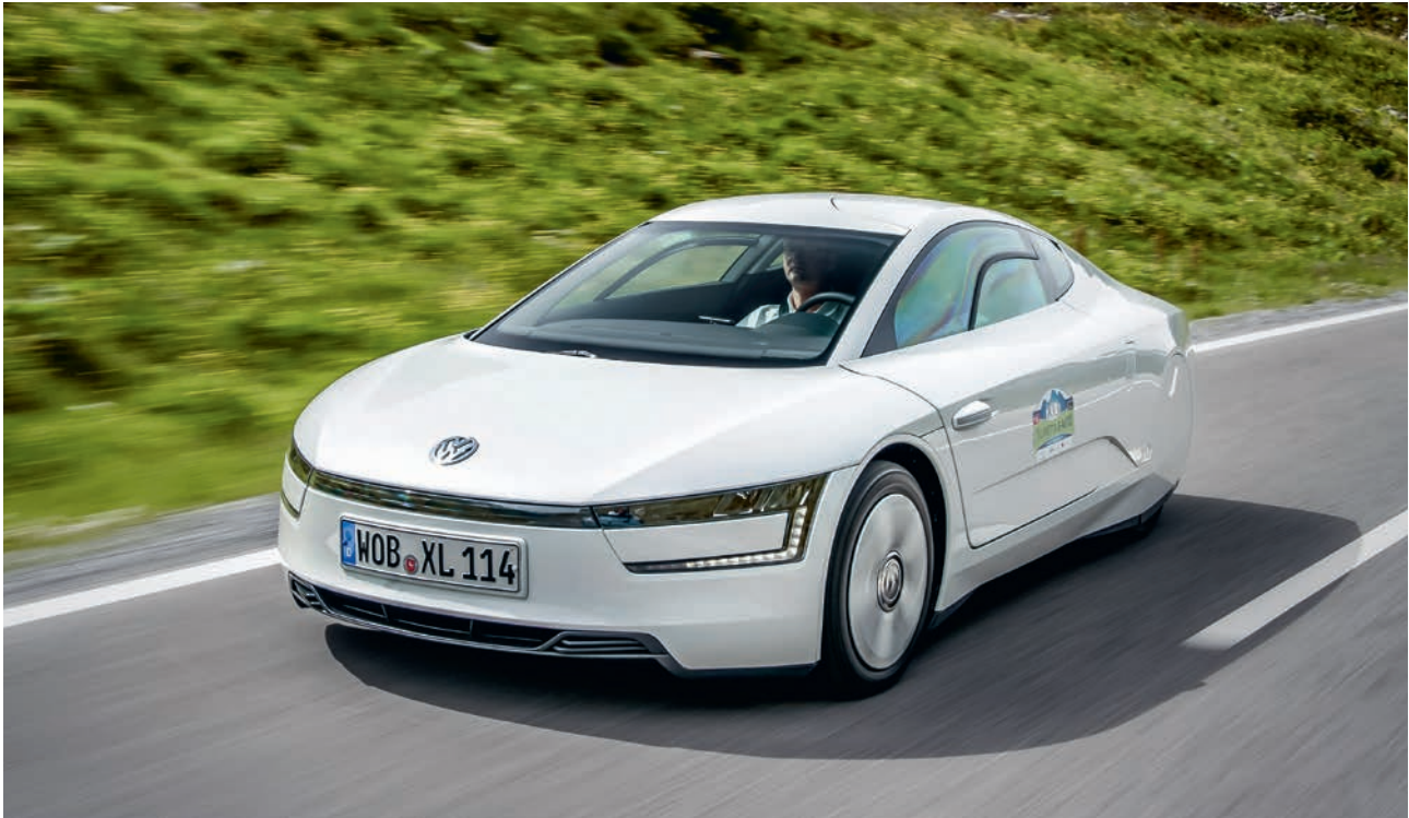
Volkswagen delivered the first XL1* in May 2014. With test cycle fuel consumption of 0.9 l/100 km, this is the world's first "1-liter" car.
