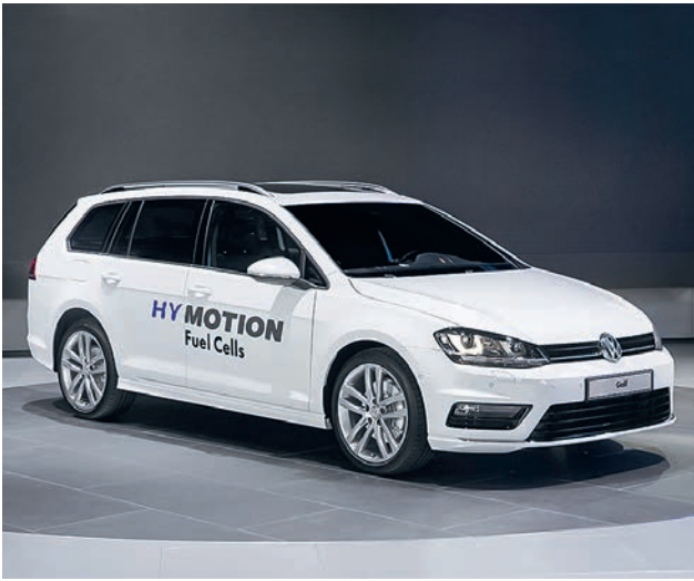
The fuel cell drive in the Golf Estate HyMotion concept vehicle runs on hydrogen and oxygen.
