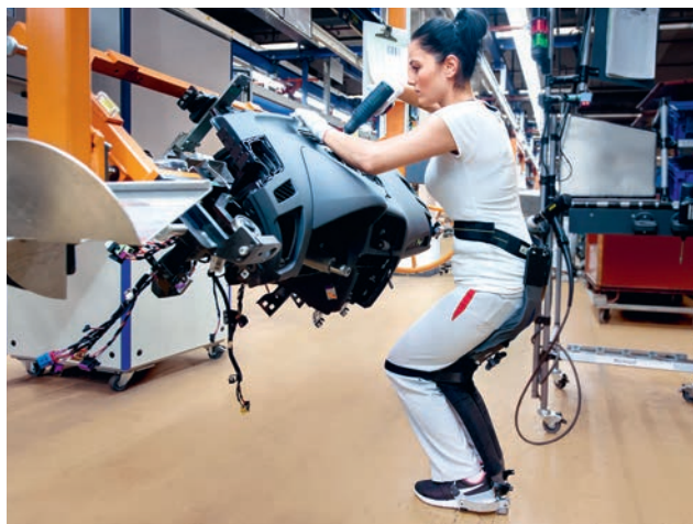
The Chairless Chair makes many assembly activities easier. This high-tech carbon-fiber construction allows employees to sit without a chair. At the same time, it improves their posture and reduces the strain on their legs.
