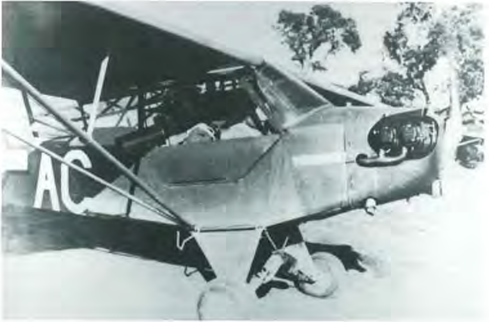
AN L-4 WITH A FAIRCHILD K-24 AERIAL CAMERA MOUNTED FOR OBLIQUE PHOTOGRAPHS TAKES OFF FROM THE ANZIO BEACHHEAD, 1944.
