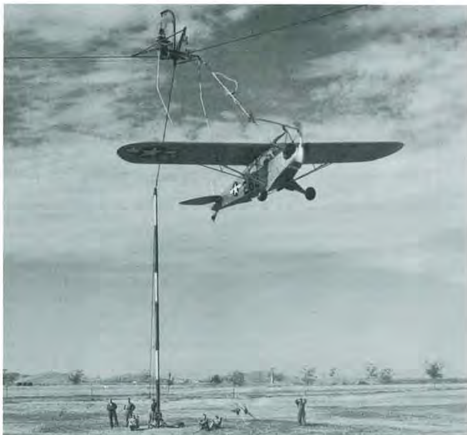
AN L-4 ON THE LAND-RIG VERSION OF THE BRODIE DEVICE AT FORT SILL
