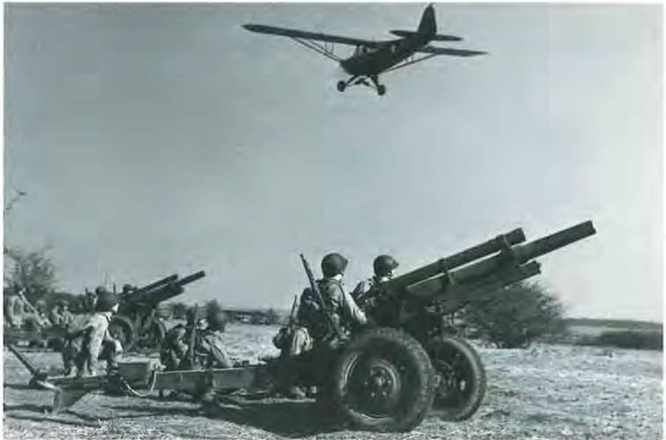
AN L-4 OF THE 29TH INFANTRY DIVISION FLIES OVER A BATTERY OF 105-MM. M2 HOWITZERS, MARCH 1943.
