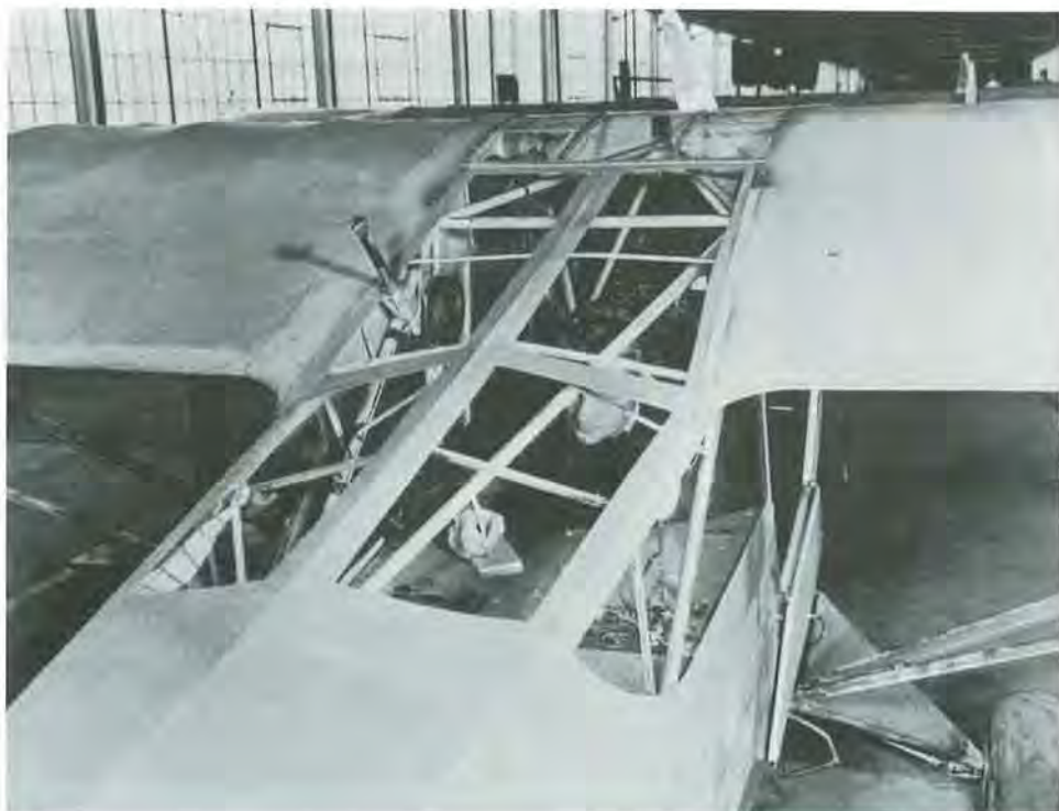
AN OVERHEAD PHOTOGRAPH OF THE YO-59A AT THE PIPER AIRCRAFT CORPORATION PLANT IN LOCK HAVEN SHOWS THE IMPROVED OVERHEAD VISIBILITY AVAILABLE IN THE MILITARY VERSION OF THE PIPER J-3 CUB, 12 FEBRUARY 1942.
