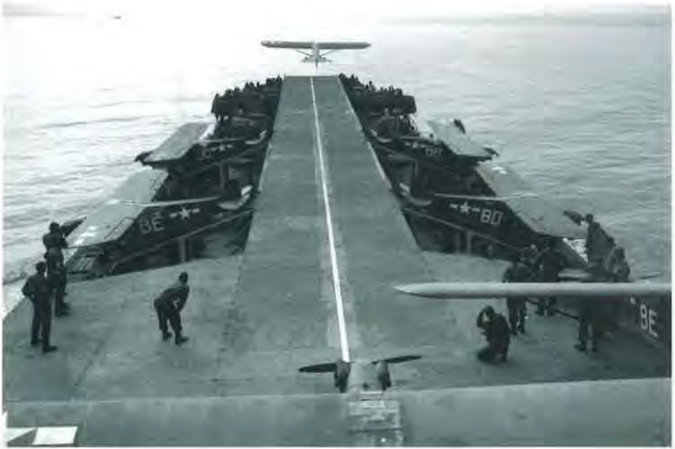
A 3D INFANTRY DIVISION L-4 CUB TAKES OFF FROM A ONE-WAY RUNWAY BUILT ON AN LST IN THE MEDITERRANEAN, JULY 1944.
