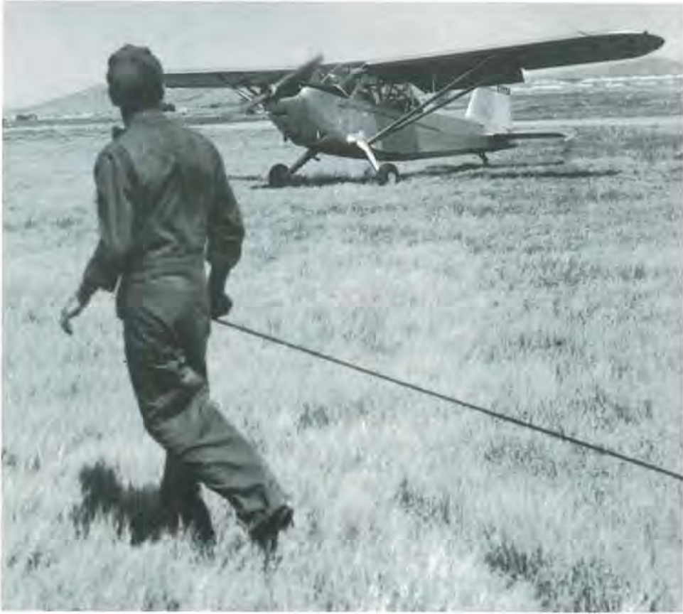
MEASURING TAKEOFF AND LANDING DISTANCES DURING THE STINSON MODEL 76 TESTS AT FORT SILL
