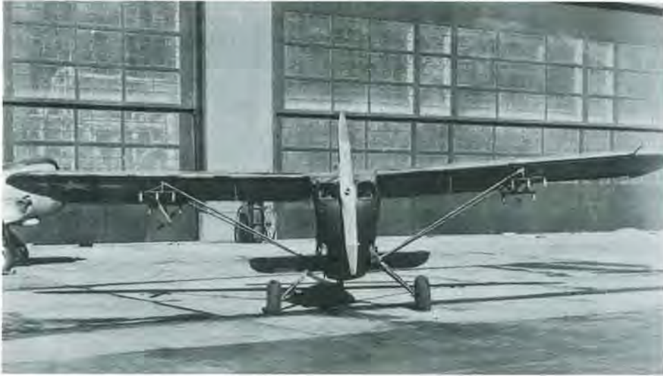
AN L-5 AT THE DEPARTMENT OF AIR TRAINING OUTFITTED WITH SIX ROCKET LAUNCHERS WITH ONE NAVY 5-INCH HIGH-VELOCITY AERIAL ROCKET IN FIRING POSITION, 1945
