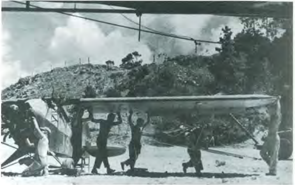
MAINTENANCE SPECIALISTS OF THE 1ST DEPOT UNIT, ARMY, ON OKINAWA, INSPECT THE ENGINE OF AN L-4 AND REMOVE A BATTLE-DAMAGED WING FOR IMMEDIATE REPAIR.
