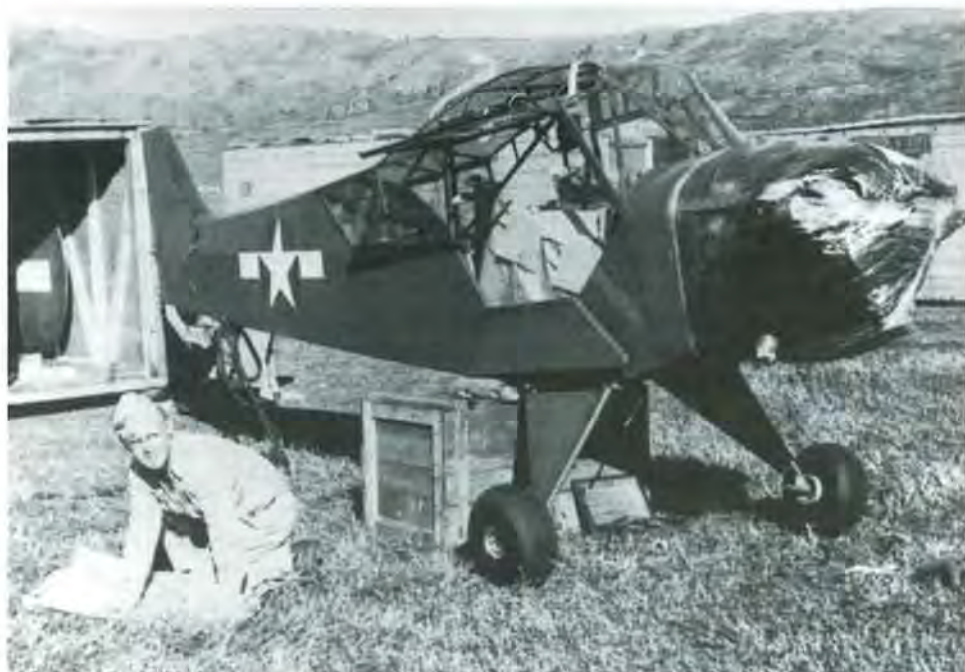
FIELD ASSEMBLY OF AN L-4 ON OAHU, TERRITORY OF HAWAII, 1943. NOTE THE OVERSEAS CRATE IN THE REAR CONTAINING THE WINGS.
