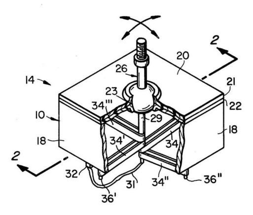
**Figure 8: The original joystick patent awarded to Stephen D. Bristow of Atari.** (U.S. Patent Office)
