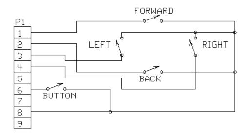
**Figure 5:** A simple circuit diagram for a basic joystick. A basic joystick can easily implemented with four switches, each of which turned on (closed the circuit so that a current would flow) when the stick is moved in the appropriate direction. (Engdal, Digital joystick connector pinouts)
