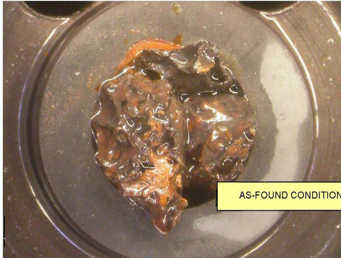
Figure 4-11: As-found Condition of Upper Trap Following Cap Removal (Lower trap had similar deposits, refer to [8])
