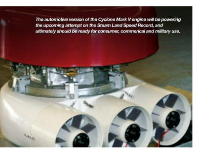
oil. In fact, one of the amazing features of the Cyclone engine is that it is completely water-lubricated—it requires no motor oil
