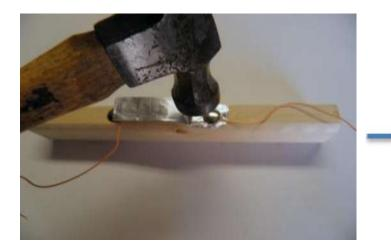
Hammer the tacks in to lock the wires in place. This completes the fan's switch.
