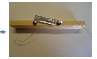
Add a second tack under the other end of the foil. Wrap a piece of wire (ends exposed) around each tack.
