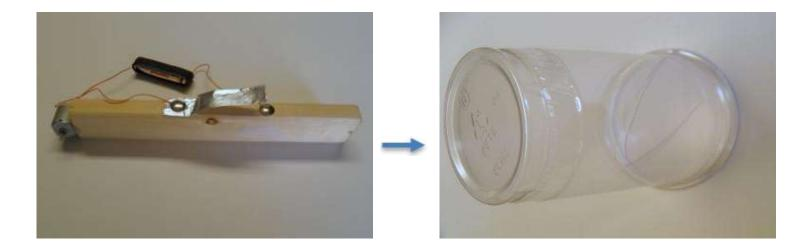
Hot glue the motor to the top of the handle. Bend the foil up away from the tack. Tape the battery to the handle. Cut an oval out of a plastic bottle or jar. This will be the fan's propeller. Cut it at an angle like shown and it will have the necessary curvature built into it.
