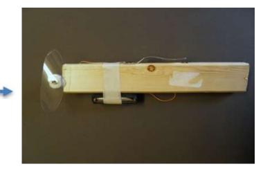
Attach the propeller to the motor shaft. Press the foil into the thumb tack to turn on your fan!
