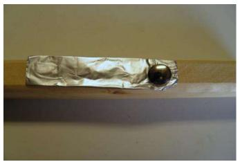
Fold the foil into a strip 2" long and the same width as the narrow side of the wooden handle. Loosley tack it in place onto the handle.
