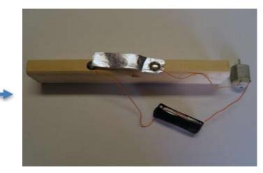
Add a third piece of wire to create a complete circuit between the tacks, motor, and battery. Wrap a thick rubber band or tape around the battery to keep the wires secure.
