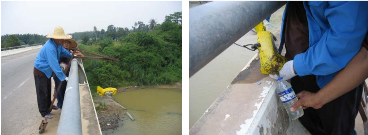
Figure 5.8 Bed Load Sampling @ Ladang Victoria (20 July 2006)
