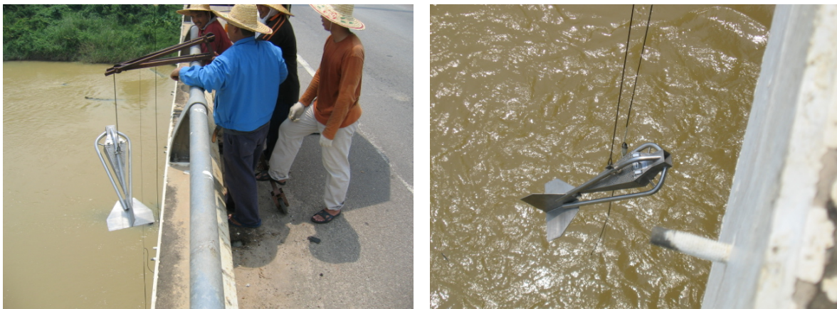
Figure 5.7 Bed Load Sampling @ Ladang Victoria (20 July 2006)
