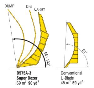
Unlike ordinary dozer blades, the Super Dozer blade has a full range of movement. Three basic positions—dig, carry, and dump—create previously unheard-of levels of efficiency. It also includes auto-dump and auto-reposition features.
