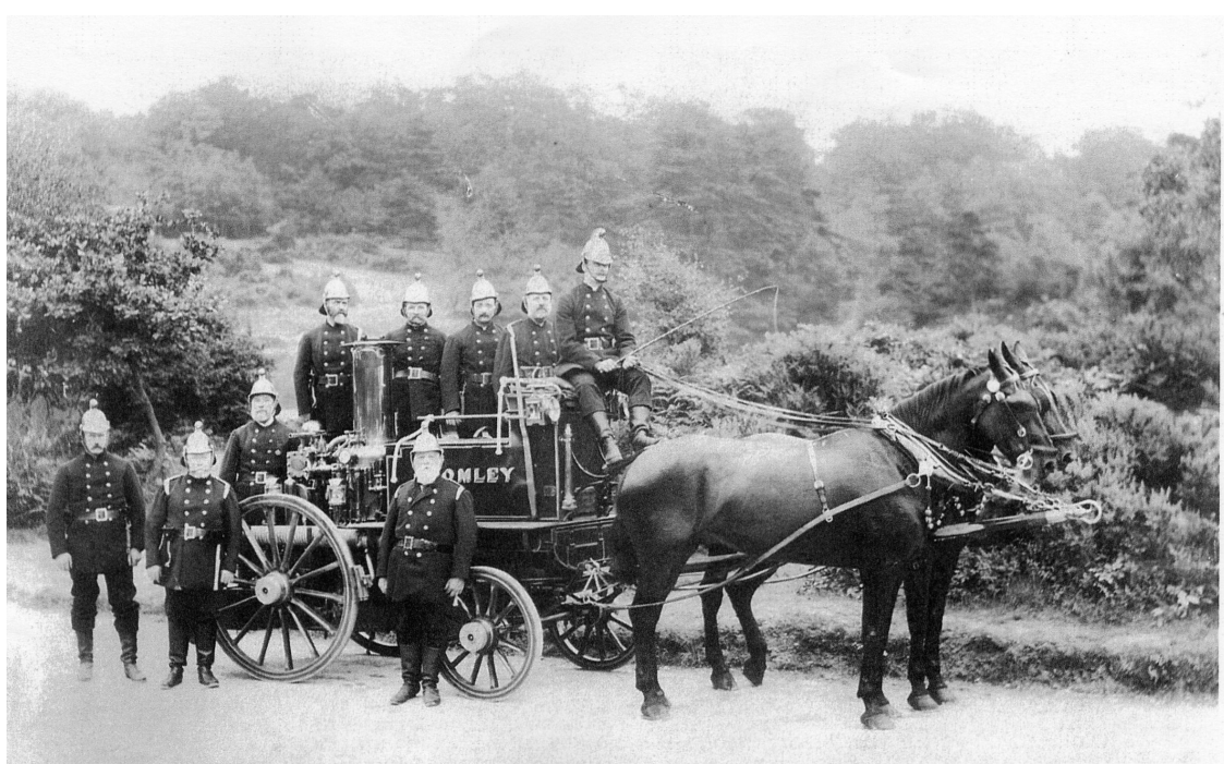
Bromley UDC bought this Shand Mason 260gpm double vertical steam pump at a cost of £430 in 1897. It was sold to Albert E. Reed & Co. Ltd for use at its Horton Kirby paper mill in 1919 and is now kept by Kent Fire & Rescue Service in a restored condition. (Kent FRS Museum)
