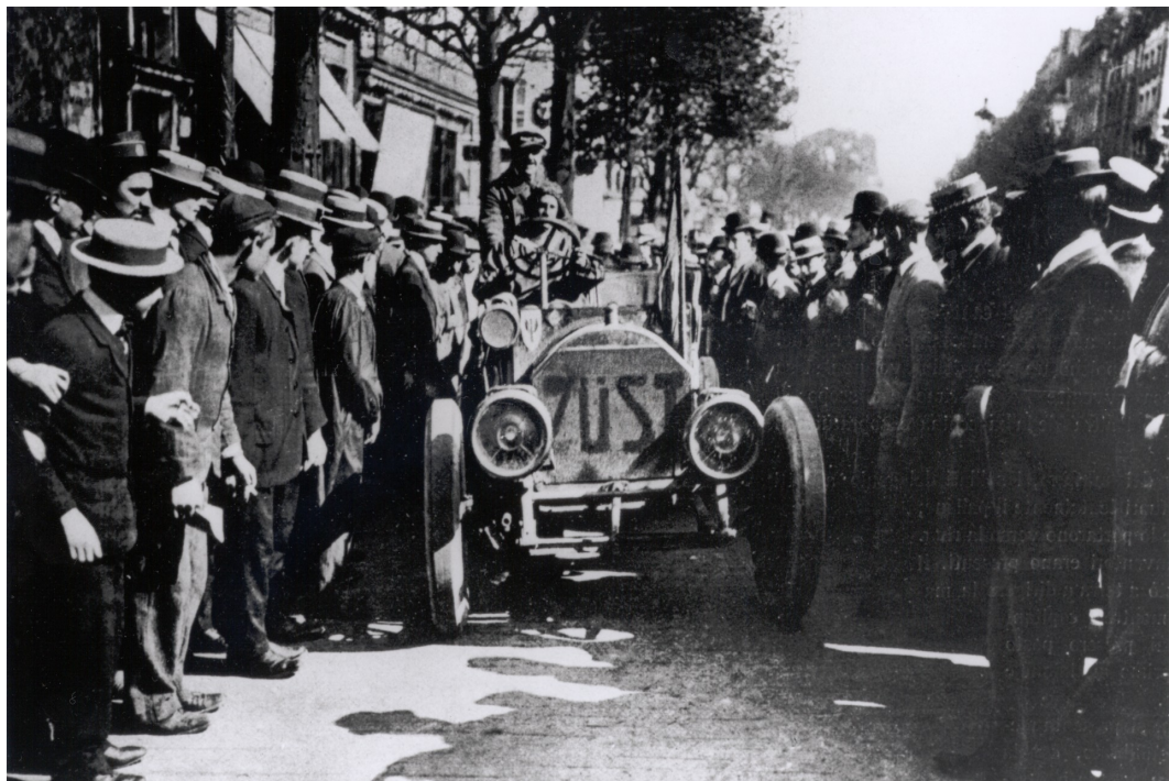
Figure 3 The Züst entering Paris, with round headlamps, one sidelamp missing, different driver's side sidelamp and no rounded cowl. The mudguards and folding canvas top are also missing. Resnick Collection, Western Reserve Historical Society
