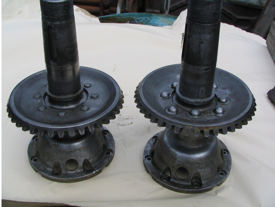
Figure 10 The rivets holding the ring gears in place, hand fabricated on the right.
