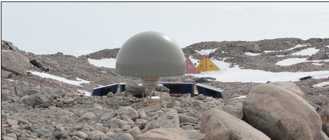
Figure 5.4: The CORS at Wilson Bluff is located on a rock outcrop beside the campsite.
