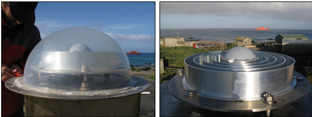
Figure 2.13: Macquarie Island ARGV GNSS antenna, dome and bracing mount
