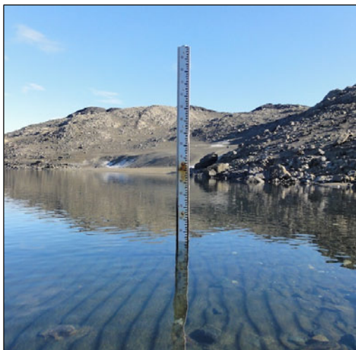
Figures 6.1: a) level staff at Deep Lake, b) calculating the height difference between the benchmark and lake level at Pendant Lake.
