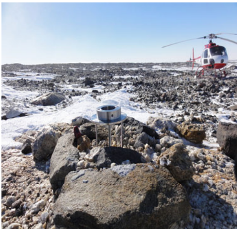
Figure 5.12: Deconstruction of the Mt Creswell CORS. Note Shim was only partially removed due to extreme cold.
