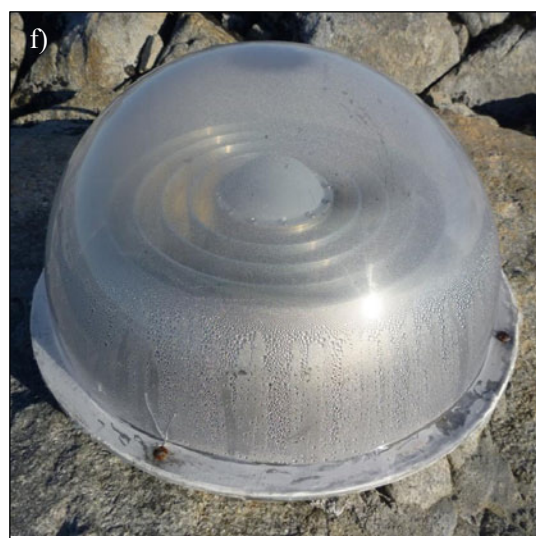
Figure 2.7: a) the Casey CORS antenna facing north, b) east, c) south, d) west, e) the equipment rack and f) antenna showing condensation and small crack.
