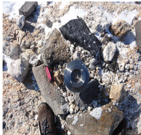
Figure 5.12: Deconstruction of the Mt Creswell CORS. Note Shim was only partially removed due to extreme cold.
