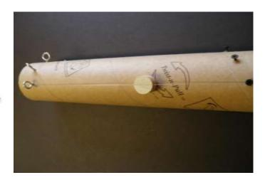
Tie fishing line between each eye screw and each wood screw. File a groove down the centers of four small pieces of wood and hot glue them to the tube under each string. These are the bridges.
