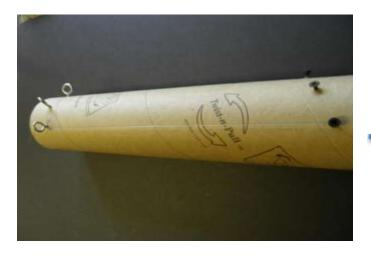
Twist the eye screws into the holes around the ring, and twist the wood screws into the holes drilled at different heights.
