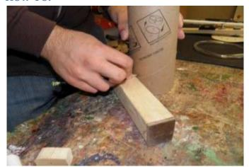
Use an object like a wooden block to draw a ring around the tube about 1.5" high.
