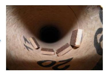
Hot glue small pieces of wood behind each hole to hold the screws more securely.
