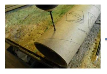
Drill a hole along the ring at each point where the parallel lines intersect it. Drill another hole along each of the parallel lines. Drill the holes at different heights so the strings will be of different lengths and produce different notes.
