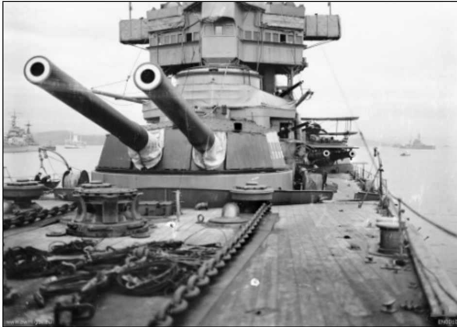
Figure 4: View along the fore deck of HMAS Australia , showing 'A' turret with 12 inch guns, 4 inch guns behind, and a two seater Sopwith 1 1/2 Strutter biplane on a platform above the port turret. (Photo: Australian War Memorial Image # EN0010)
