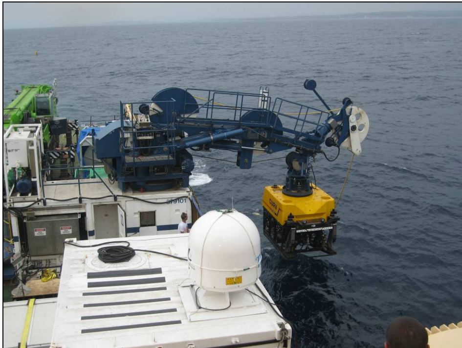
Figure 29: ROV USN CURV 21 being launched for a similar photographic survey of the M24 Japanese midget submarine (Photo: David Nutley 2007)
