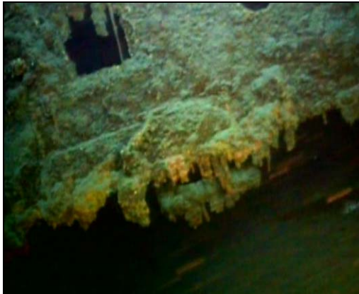
Figure 70: Rusticles on starboard bow section (Photo: DMS 2007)
