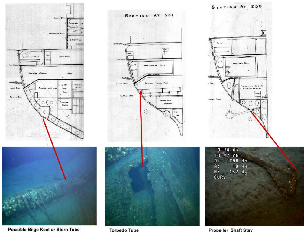
Figure 67: Stern features identified from HMAS Australia (Image: Brad Duncan after DMS 2007 and Beandford n.d. - AWM Plans)
