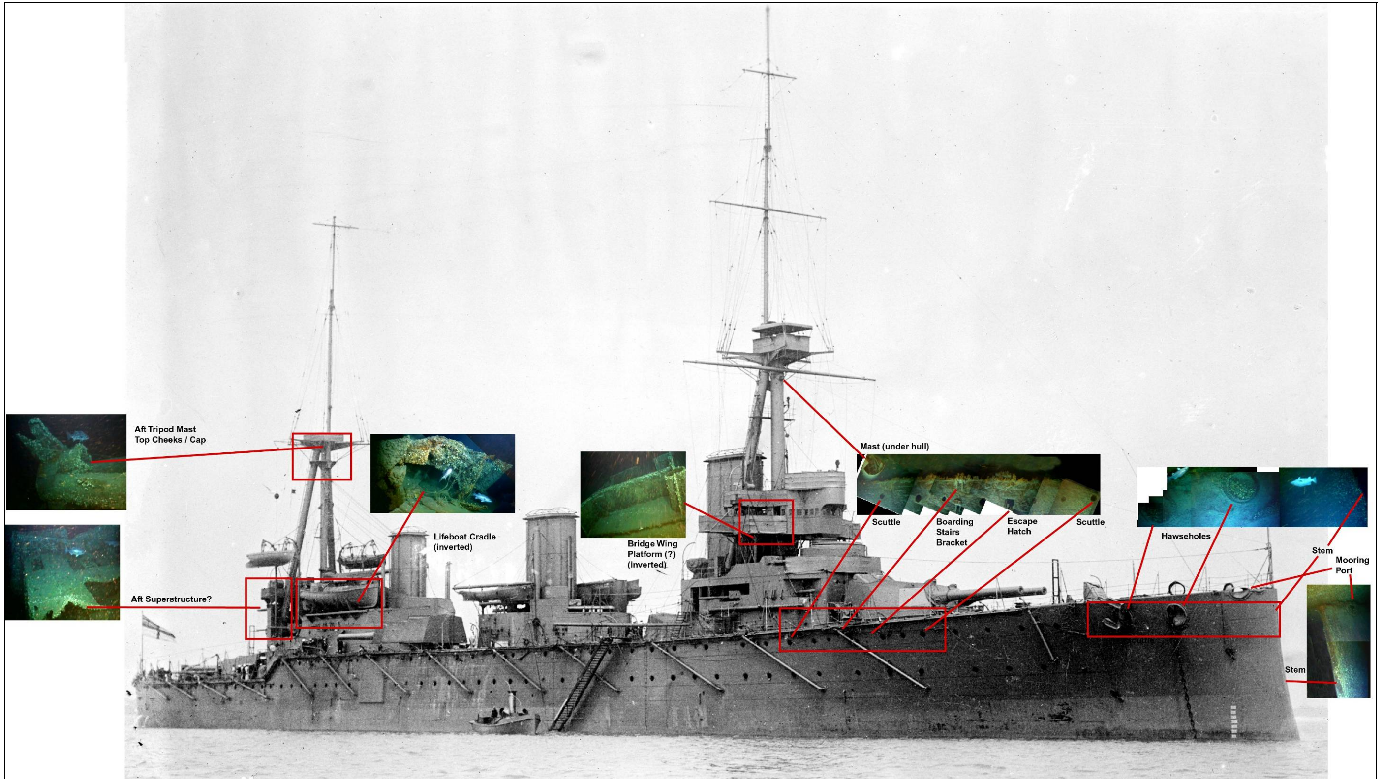
Figure 68: Features confirming the identity of HMAS Australia (Image: Brad Duncan after DMS 2007)
