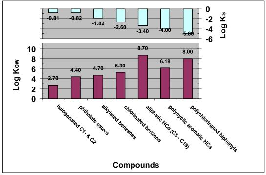
Figure 4. Median values of *K<sub>OW</sub>* and *K<sub>S</sub>* of representative compounds (Adapted from Schwarzenbach et al., 1993)
