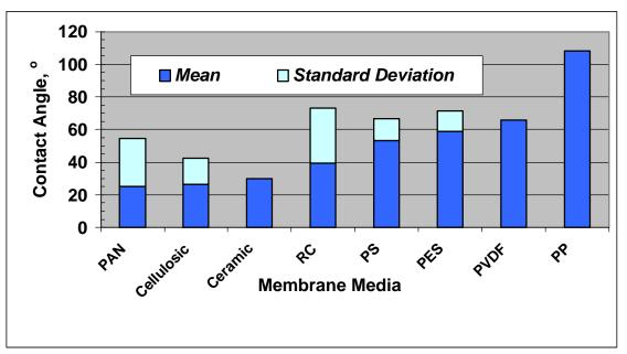
Figure 3. Hydrophobicity of various membrane media (data from Cheryan, 1998): PAN- polyacrylonitrile, RC-regenerated cellulose, PS – polysulfone, PES – polyethersulfone, PVDF – polyvinylidene fluoride, PP – polypropylene
