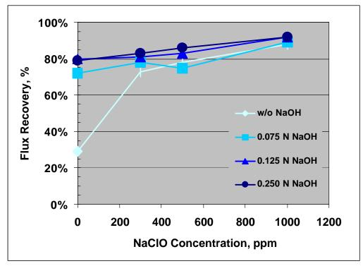
Figure 8. Effects of NaOCl and NaOH concentrations on cleaning of hollow fiber samples taken from Site A.
