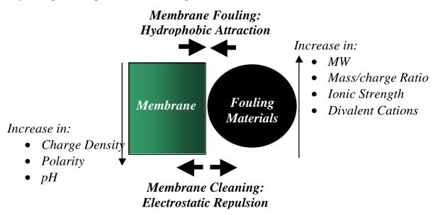
Figure 6. Conceptual Model of Membrane Fouling and Cleaning
