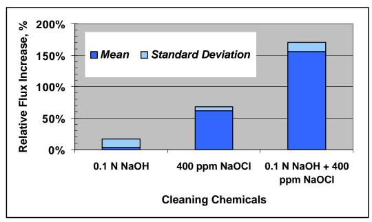
Figure 7. Comparison of effects of cleaning chemicals on flux
