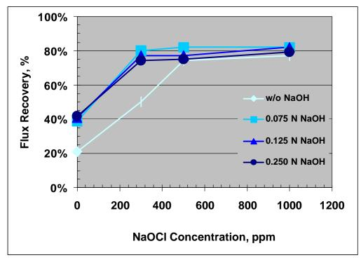
Figure 9. Effects of NaOCl and NaOH concentrations on cleaning of hollow fiber samples taken from Site B.
