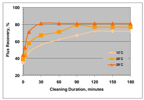
Figure 10. Effect of temperature on chemical cleaning of hollow fiber samples Cleaning solution: 5,000 ppm NaOCl + 0.25 N NaOH
