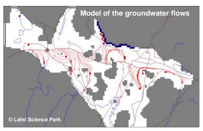
example, the amount of groundwater pumping as well as flows of groundwater. The model has been based on data collected from the soil and groundwater during the past decades. Some new gravity scalings and drillings have been made and some new observation tubes installed for this modelling process. The modelling has been carried out by using finite difference -method based on MODFLOW-calculation code. Furthermore, PMWIN- and PMPATH- programmes have been used in data input and illustrations.
