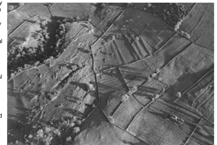
The hillocks at the Old Ash Mines above Northern Dale near Wensley are a classic example following parallel veins, which take on added importance because of their relationship to ancient agricultural earthworks. Unfortunately, some of those at the upper centre of the photograph have been badly damaged since this was taken. Further hillocks are hidden in the woodland of Northern Dale to the left, which are associated with archaeologically important ancient pipe workings (Derrick Riley collection).
