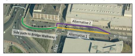
Figure E12: Sidepath proposal for 5th Street approach to south walkway of the Ben Franklin Bridge; shows Alternative 1 on 5th Street south of Race Street. (credit: Bicycle Coalition of Greater Philadelphia)
