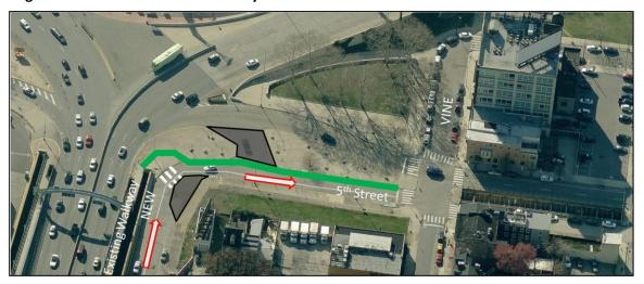
Figure E11: Alternative bikeway approaches to south walkway of the Ben Franklin Bridge
