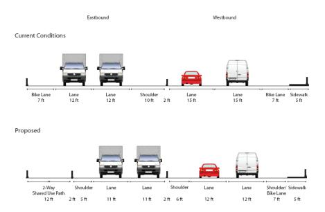
Figure 23: Recommended Grays Ferry Bridge Bikeway
