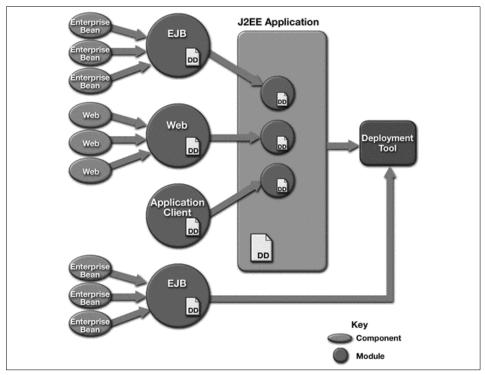
Figure 3-5 J2EE packaging and deployment overview
