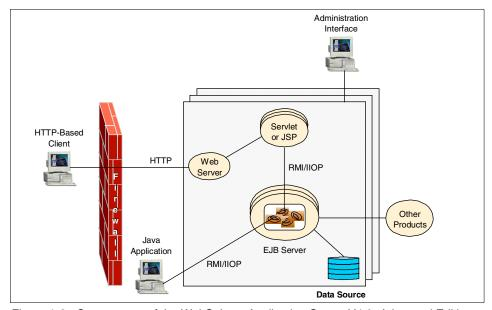
Figure 1-3 Components of the WebSphere Application Server V4.0, Advanced Edition
