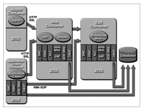
Figure 3-2 J2EE components, containers, and services
